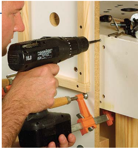
Mount the adjustable carriage to the table. Clamp the carriage in place so that it sits perpendicular to the tabletop. Drill holes for carriage bolts and steel dowels and are tightened in place with threaded handles.
