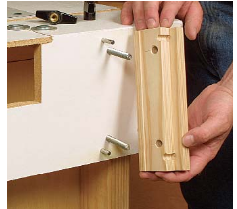
Clamp blocks secure the adjustable carriage. The clamp blocks fit over the carriage bolts and steel dowels and are tightened in place with threaded handles.
