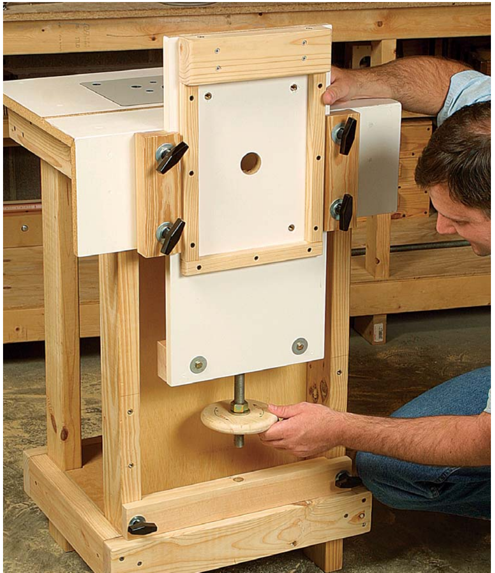
Two ways to set the adjustable-carriage height. The position of the carriage can be finely adjusted with a wheel. Gross adjustments are made by moving the lower adjustment rail to different positions on the table legs.
