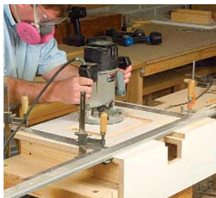
Framing squares ensure a 90° fit. Clamp the top and back to two Speed Squares, and then clamp the mitered joint.
