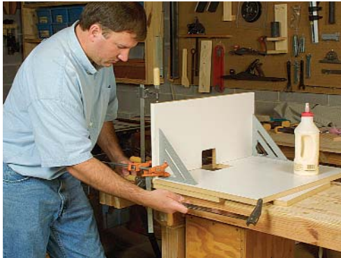
Framing squares ensure a 90° fit. Clamp the top and back to two Speed Squares, and then clamp the mitered joint.
