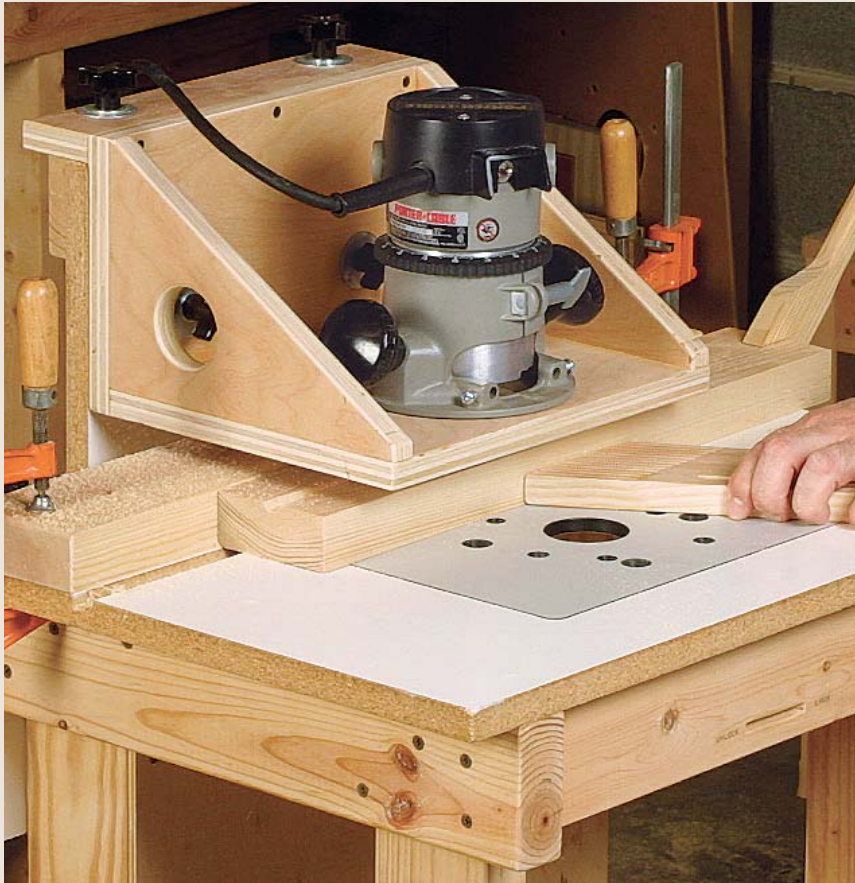
An overhead router carriage holds the router upright above the table, allowing the flat side of a workpiece to be referenced on the tabletop.
